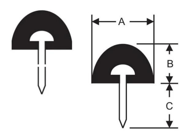
RPM's rubber recessed bumpers are used to protect doors or truck bodies from damage. They are also used as feet for large vibrating equipment.
