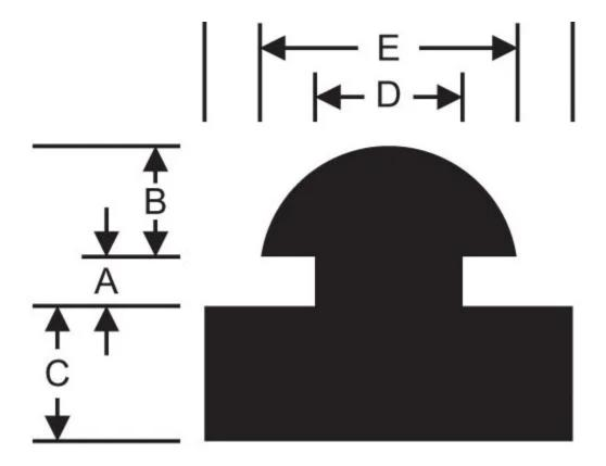
RPM's rubber recessed bumpers are used to protect doors or truck bodies from damage. They are also used as feet for large vibrating equipment.
